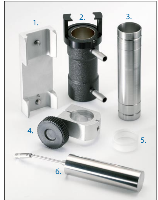
Detail of UL Adapter: 1. Locating Channel Assembly, 2. Water Jacket, 3. Chamber Tube, 4. Collar with thumbwheel, 5. Tube End Cap, 6. Spindle with universal coupling
